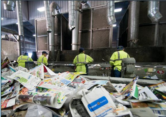
Workers on the sorting line in Vallejo carefully inspect recyclable materials. They remove any improper or contaminated items before materials are packaged for shipment.
